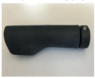
These grips have a fixation ring in the front. Bring the grip together with the ring on the handlebar. Choose the preferred position and fixate the ring by tightening the ring with the screw (inbus 2,5). The gap in the fixation ring should be completely closed.
